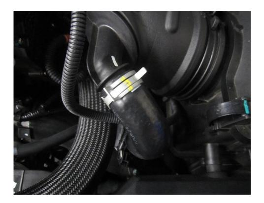
4. Moving to the other end of the OE intake Pipe there are two breather hoses that need to be removed, these too have spring hose clamps that just need to be compressed like step 3 to remove the hoses. Once this is complete undo the 10mm hose clamp attaching the intake hose and joiner to the turbo elbow, you will now be able to remove the air box and intake pipe together as one part.
