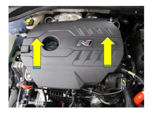
8. With the engine cover removed you will be able to access the engine cover locators, the locator in the picture below must be removed with a 10mm spanner.
