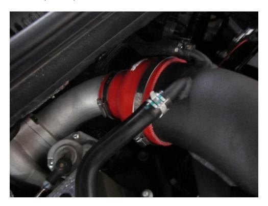
**11.** Re fit the engine cover locator through the intake pipe bracket. Now you can adjust the silicone hose and tighten it in position.
