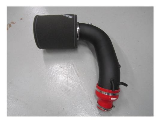
10. The intake can now be positioned in the engine bay, attach the silicone hose to the turbo elbow. Don't tighten the hose clamps at this point.
